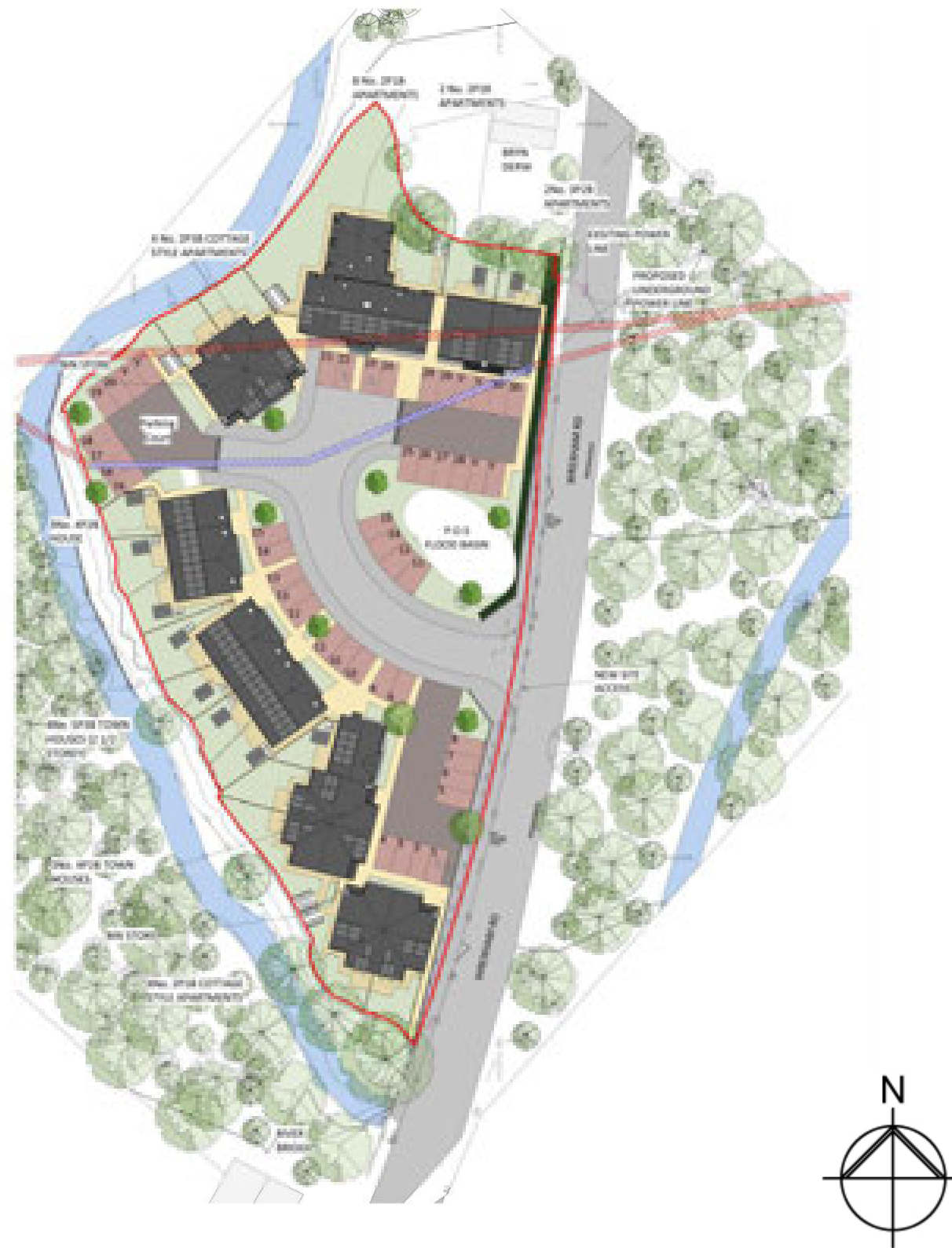
Image 01 - Site Layout showing general disposition of dwellings. Roof plans show location of PV panels integrated into the slate roofscape and orientated to maximise solar energy generation.
